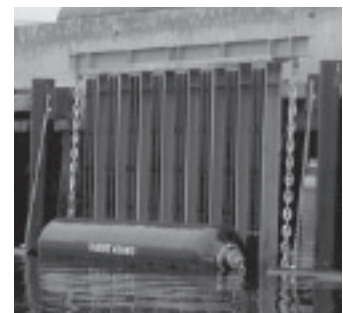
attachments A floating fender with fixed chain attachments
